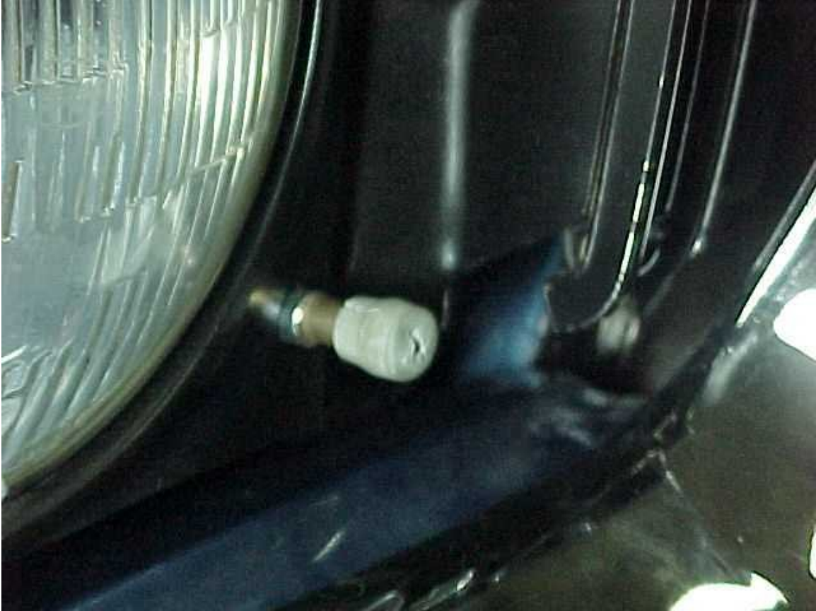
Picture showing the steel spacer cut down to ¼" height, the bronze bushing and the rubber sun visor tip. The screw is inside and cannot be seen.
