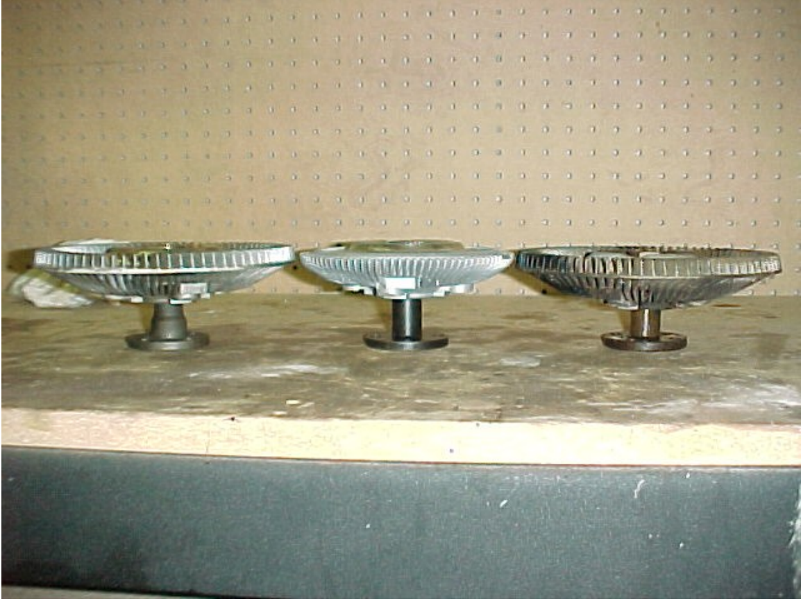
From the left: C9SE-B, C9WE-A and C80E-A. The one on the right is original 390 /427 / 428CJ. Notice all have holes rather than slots in the flange.
