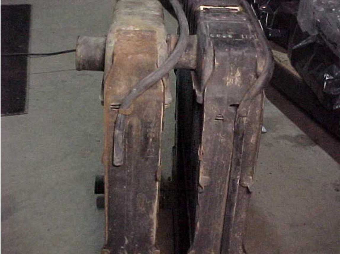
More differences occur on the side. The 1969 radiator (left) has C9ZE- E1 and a relocated overflow tube clamp. The 1968 unit has other subtle differences in the side straps, little indentations on the front and rear stiffening flange not seen in the 1969 units. If this were a C8ZE-M radiator for 1969 or 1970 the C8ZE-M designation would be seen.
