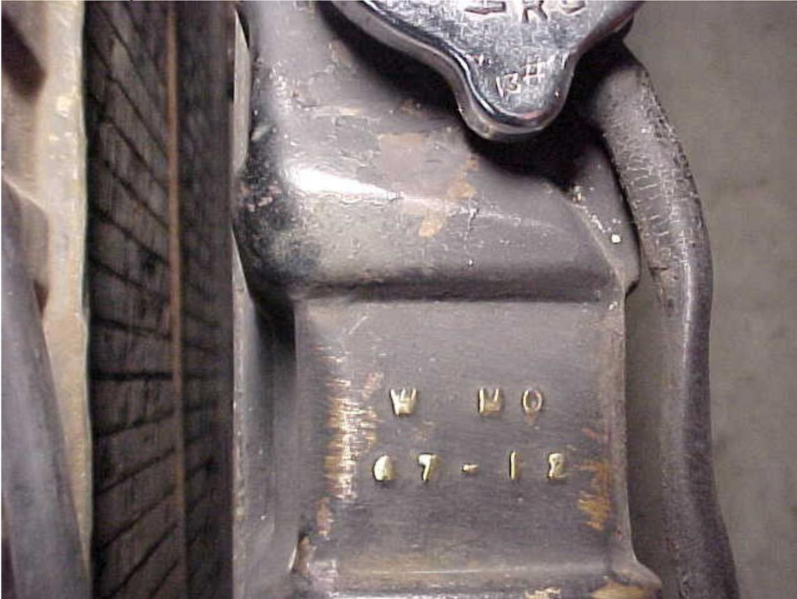
This picture (above) shows a date code on a 1968 Cougar radiator made in December 1967. The top radiator clamp hides this area when the unit is installed in the car.
