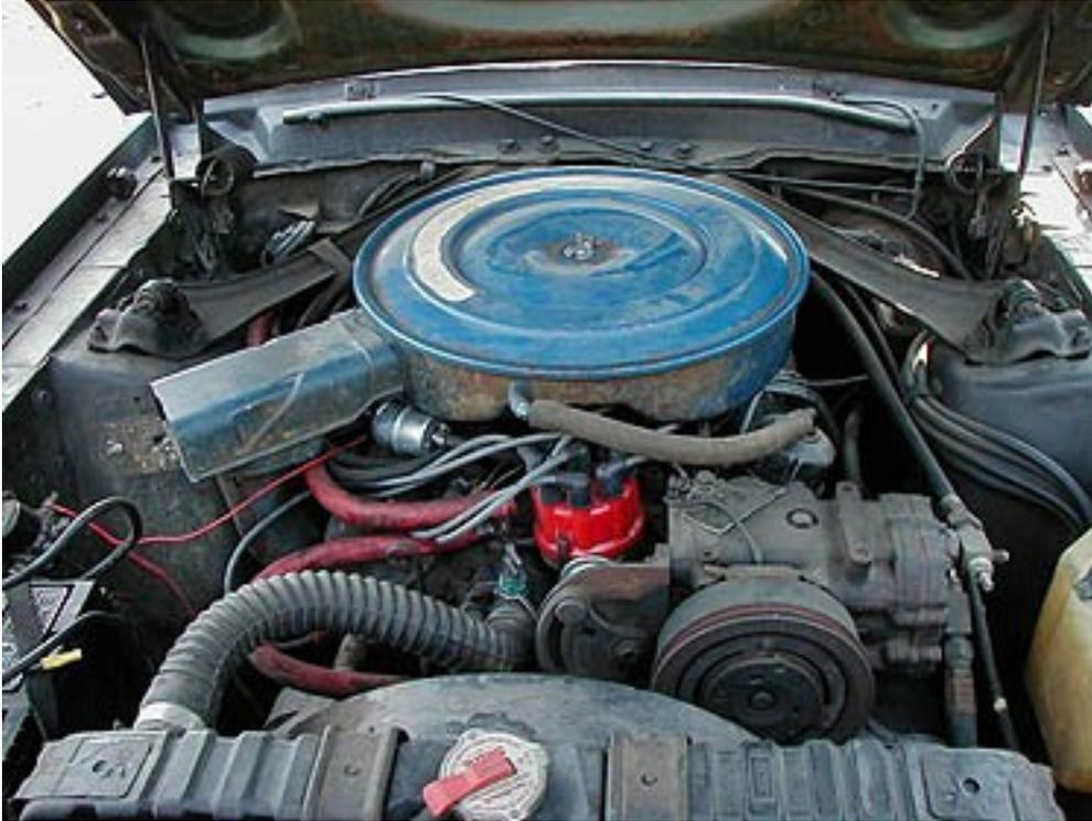
This shot is of a radiator installed in a '68 Cougar with 302 engine. Notice the clamps holding the radiator in place on either side of the cap, this is actually one piece that bolts to the radiator core support near the hood latch assembly.
