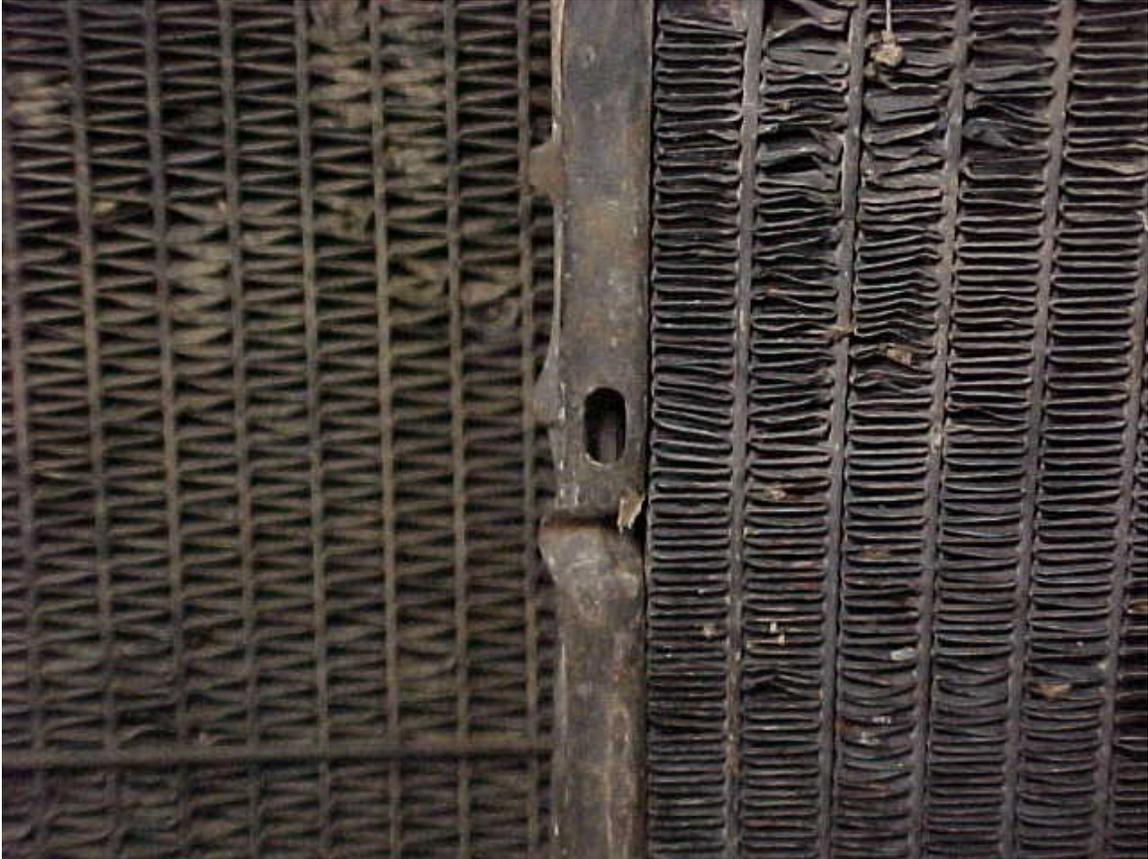
A major difference between 1968 radiators and 1969 – 70 radiators is the fin design. Ford engineers evidently found gains from increasing airflow by using fewer fins with the same tube size and spacing in the 1969 – 70 units. The 1968 unit on the right has a much denser fin spacing arrangement which would give greater surface area but hurt airflow especially as the fins became clogged with corrosion or debris over the years.
