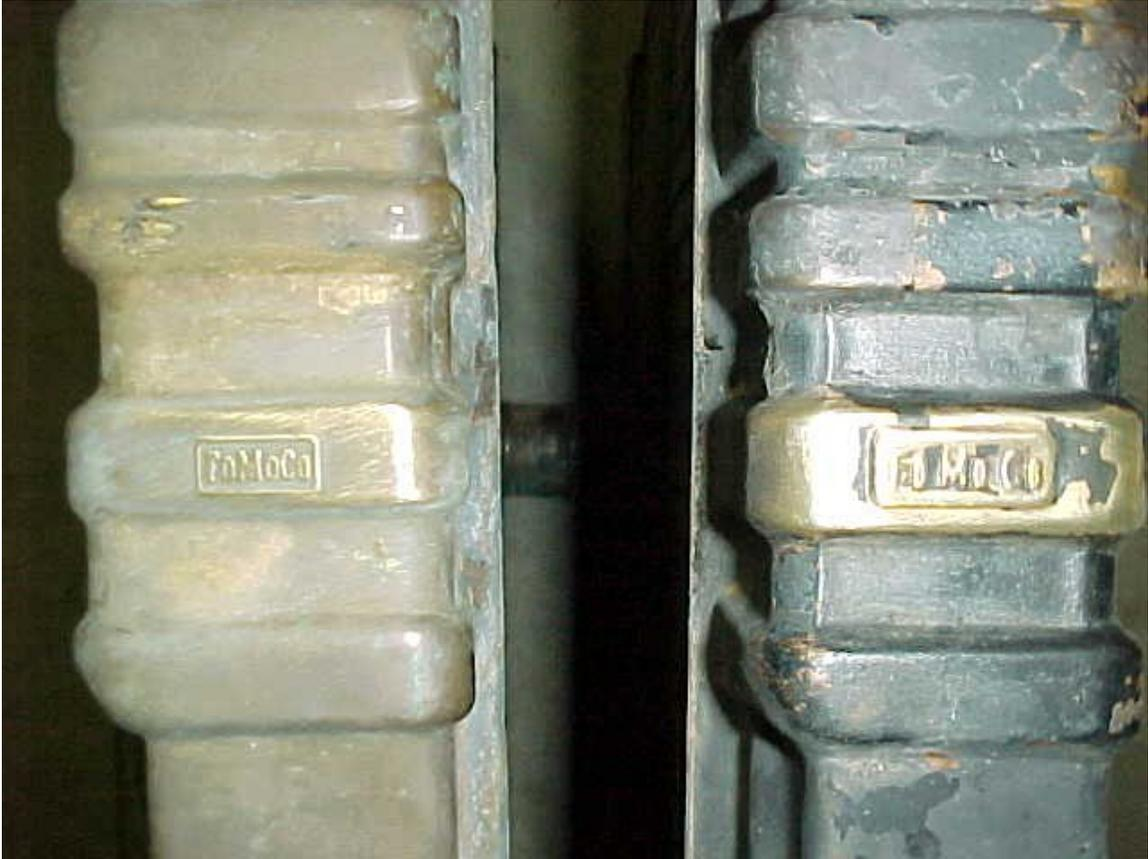
Here (above) is a comparison view of the 1969 (left) and 1968 (right) FoMoCo imprint. Notice the 1968 stamping is much larger. These marks are on the driver side of the radiator, forward would be to the right in this view.
